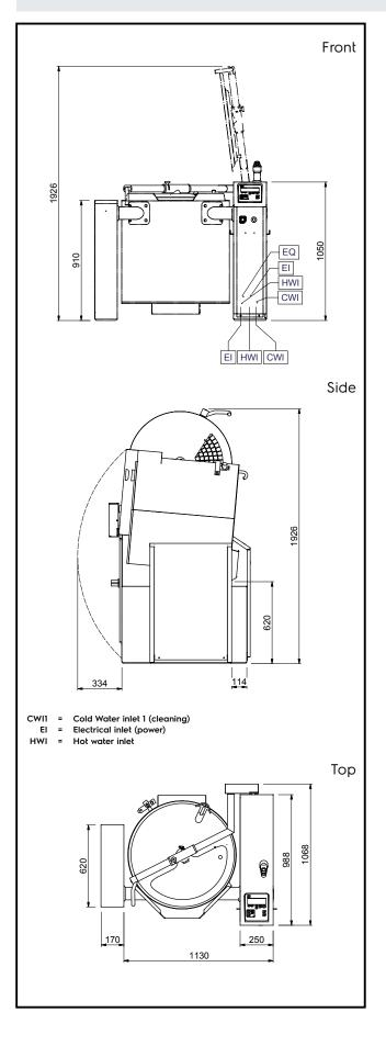
High Productivity Cooking Smart Electric Boiling Pan 150lt, 600mm tilting height
